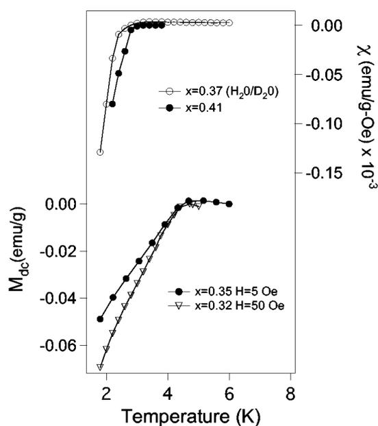
**Figure 1.** Zero-field cooled dc magnetization and susceptibility measurements of the two samples used in the NPD and ED experiments.
