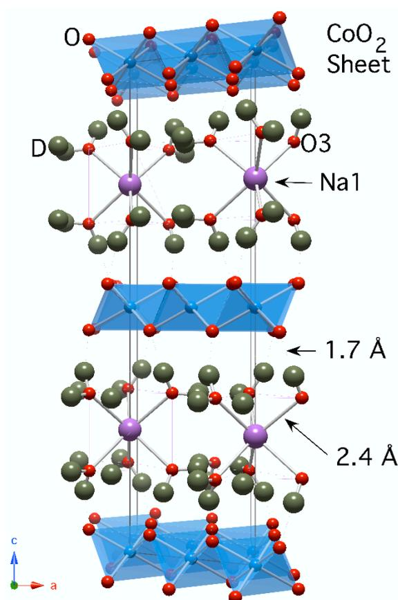
**Figure 4.** A three-dimensional representation of the structure of  $\text{Na}_x\text{CoO}_2 \cdot y\text{D}_2\text{O}$  obtained from our Rietveld analysis. For simplicity we show only the Na1 site with the  $\text{D}_2\text{O}$  molecule centred at O3. The Na–O3 and D–O(–Co) bond lengths are shown.
