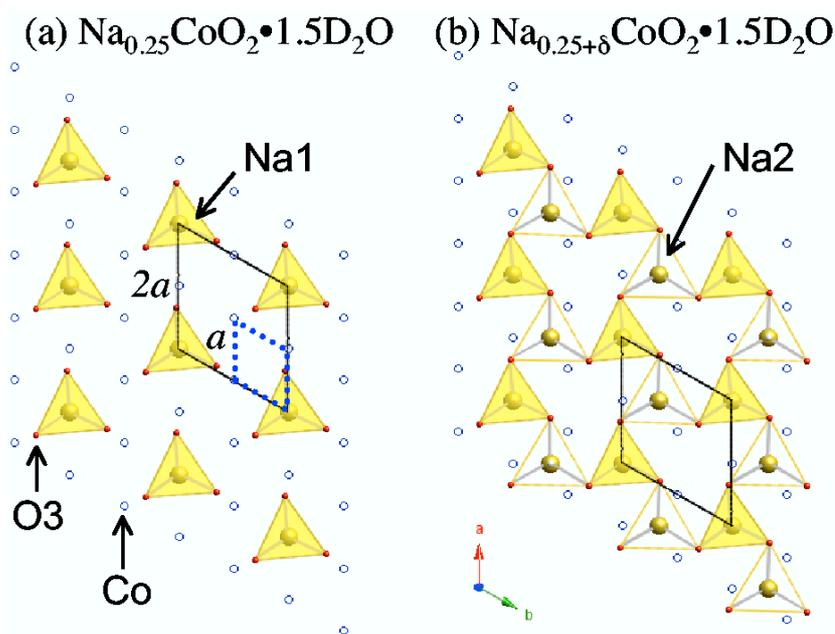
**Figure 5.** Projections of the Na-D<sub>2</sub>O layer down the *c*-axis. The NaO<sub>6</sub> triangular prisms centred on Na are highlighted. The  $2a \times 2a \times c$  unit cell is shown in solid lines and the  $a \times a \times c$  cell as dashed lines. The doubling of the unit cell is evident from the position of the Na sites. D atoms are omitted for clarity. (a) The idealized  $x = \frac{1}{4}$  structure. (b) A model for the  $x = \frac{1}{2}$  structure with the Na2 site filled.
